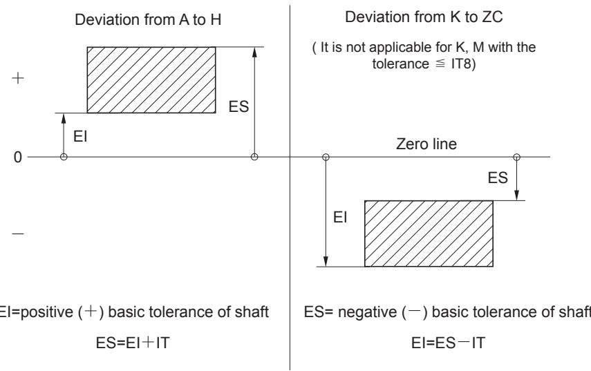
For example: for a hole with diameter 3 mm and tolerance H7, we can find that the lower deviation  $EI=0$  in relation to H7 from the basic tolerance table, and the standard tolerance  $IT=10\mu m$  corresponding to H7, thus the upper deviation  $ES=EI+IT=10\mu m$ . Therefore the hole fitting dimension is  $\emptyset 3_{0}^{+0.01}$  mm.
