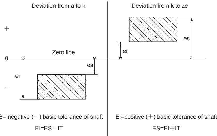
The hole lower deviation( $EI$ ) and upper deviation (ES) can be obtained by basic tolerance and standard tolerance (IT) of hole.
